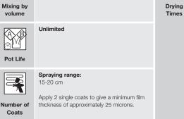
Allow to dry for 3-5 minutes between coats At 20°C: Recoatable after 10-15 minutes (depending upon film thickness)
